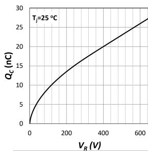
Fig. 4 Capacitive Charge vs. Reverse Voltage
